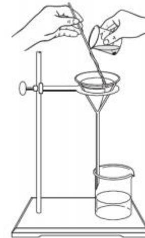
Figure 2. Proper filtering technique
